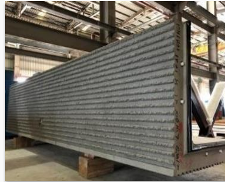
Precast exterior wall (rubber mold concrete)
